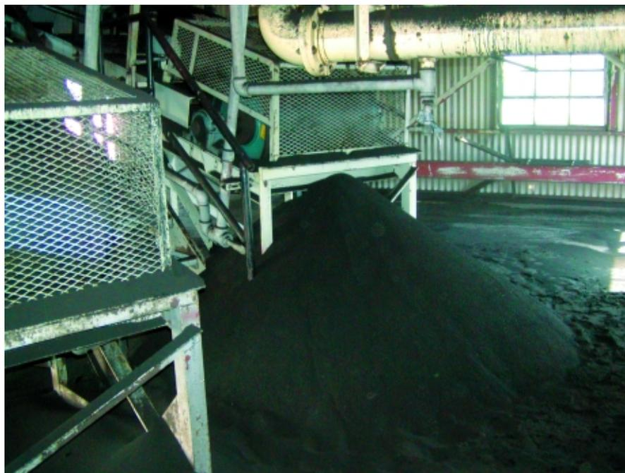
**1. Debris dump.** An extreme case of PRB coal accumulation at the tail of a conveyor not designed for PRB coal. Courtesy: Utility FPE Group Inc.
