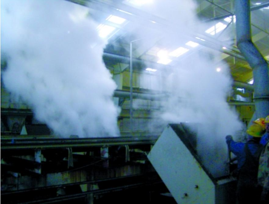
**2. Smoke means fire.** Immediate response is required when an odor of coal roasting or burning is detected as coming from a silo, bunker, or hopper. Delays in taking action only allow the rate of burning to increase. *Courtesy: Utility FPE Group Inc.*
