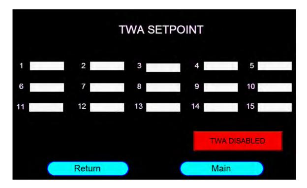
The Time Weighted Average (TWA) Set point Screen allows the user to change the Set point of each monitor's TWA Alarm. The TWA is a weighted average spanning over a user specified time. MSHA tested their time for 8 hours (480 minutes). If the monitor's TWA level is above the assigned Set point the TWA Alarm will be active. The TWA Enable/Disable button turns on and off the TWA Monitoring system. The Enable/Disable button lets the user navigate to the TWA settings page from the Main Menu.
