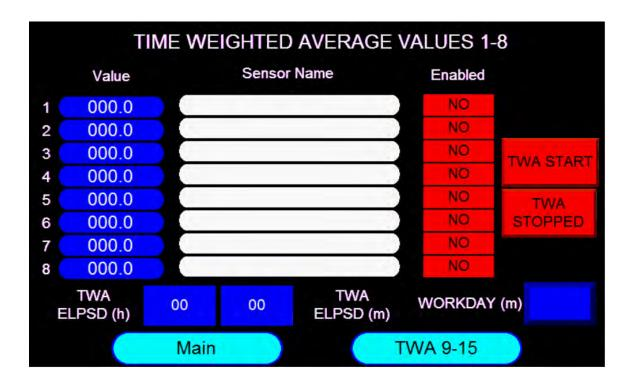
The Time Weighted Average Value has two pages. One for monitors 1-8 and another for monitors 9-15. These pages display The TWA value, sensor name, and time elapsed. These pages let the user change if the TWA is on or off, which individual monitors are enabled or disabled, and the ability to change the Workday time in minutes.
