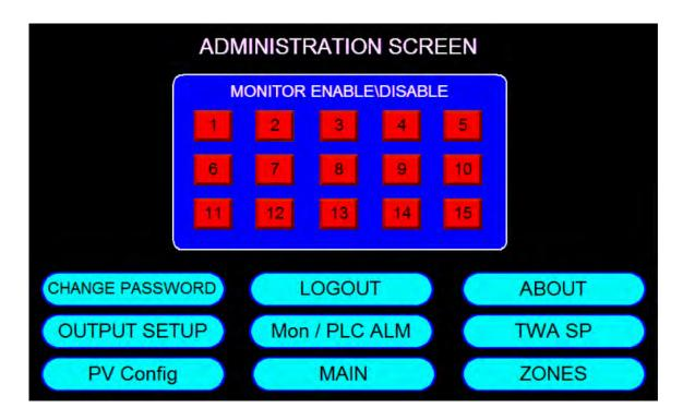
The Admin Screen has many functions. In this screen the user can enable/disable gas monitors, change the password, and navigate to multiple other screens. The user can access the About Screen, Output Setup Screen, Mon/PLC Alarm Screen, TWA SP Screen, PanelView Configuration Screen, Zones Screen, and go back to the Main Screen.
