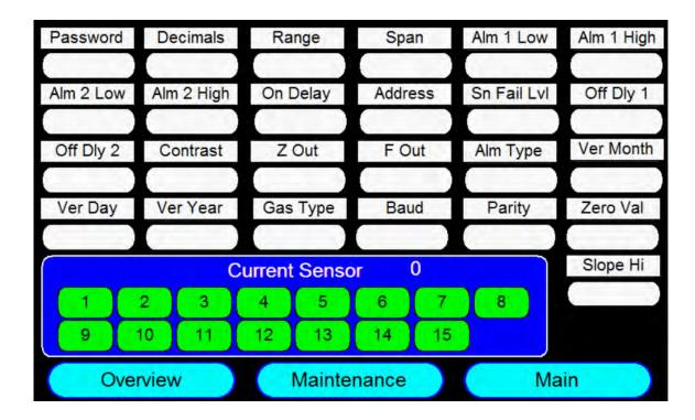
The Sensor Data screen is used to single scan all of the registers available in the CX/CN series gas monitors. To change the "Current Sensor" use the green digit buttons labeled 1-15 to select a different gas monitor. The Number shown to the right of "Current Sensor" is the sensor that has been read via the Modbus/RS485 network.
