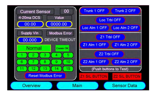
The Maintenance screen gives the user the ability to view individual gas monitor's information and test the Alarm and Trunk Outputs manually.
