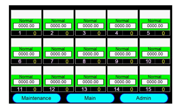
The Overview Screen is segmented to into larger gas monitor groups to allow an overview of the gas detection system
