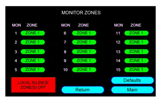
The Zone Screen is where the user is able to change the zone assigned to each monitor. To change the zone that a monitor is assigned to, press the zone button labeled as "Zone 1" or "Zone 2". Not all monitors have to be in the same zone. The monitor will not be available to change the zone unless the monitor is enabled on the Admin Screen.
