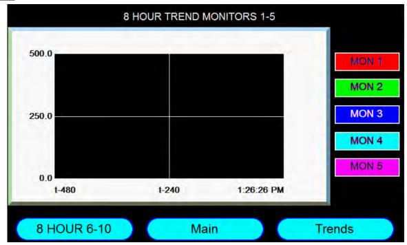
The Trends screen is a graphical representation of the sensor reading over a set period of time. The X-axis represents the sensor value. The Y-axis is represented as the TWA time. Each trend screen displays five monitors at a time. Each monitor is color coded as red, green, blue, cyan, and magenta with a legend on the right hand side so show each monitor address.
