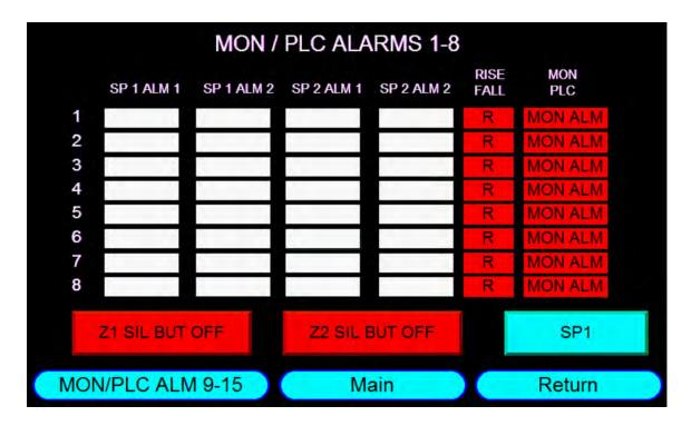
The Mon / PLC Alarm Screens let the user specify the two different Setpoints for each alarm, switch the monitors between Rising and Falling, change the alarms to activate from the Monitor or the PLC, and shows if the Input silence buttons are latched.
